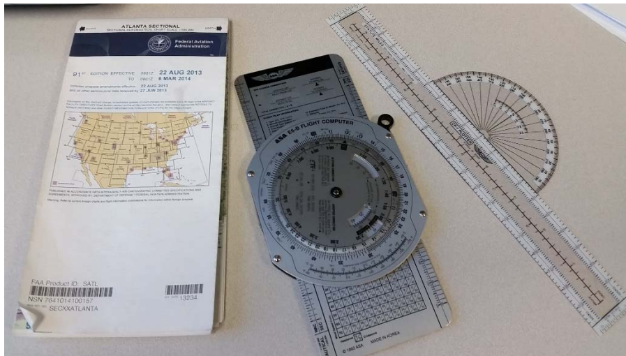
Figure 1. Sectional chart, E6B flight computer, and navigation plotter: traditional flight planning tools. (Photo credit Babb 2016.)
