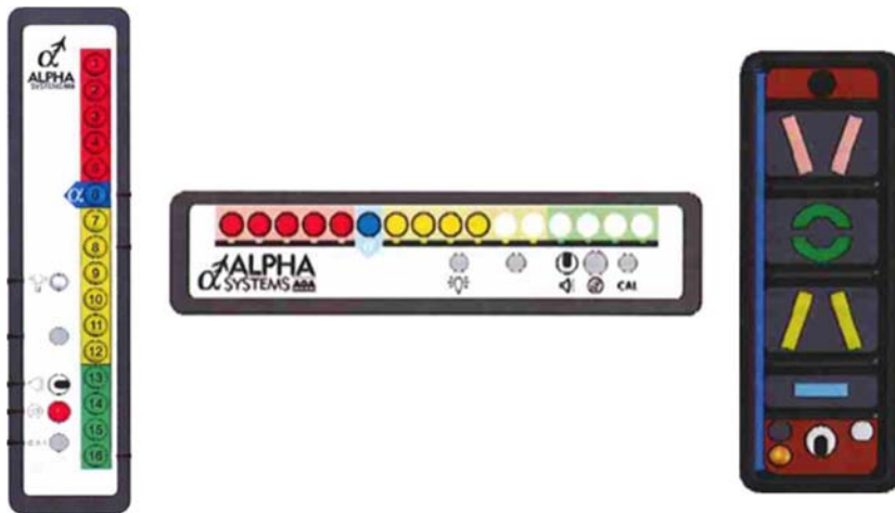
Figure 1: The three AOA indicators used in the study. Vertical bar, horizontal bar, and legacy indicators. Adapted from Alpha Systems, (2010).
