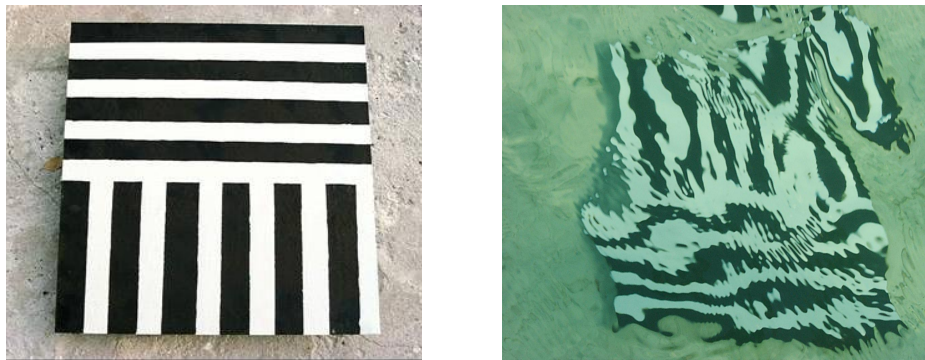
Figure 1. Line image target above (left) the water surface and below (right) the water surface. The water depth of the submerged target is approx. 1.5 m depth with winds less than 5 knots demonstrating the influence of small gravity and capillary waves on bottom feature and target recognition and identification. The methodology demonstrated is used to simulate or retrieve such features and targets from synthetic hyperspectral imagery.
