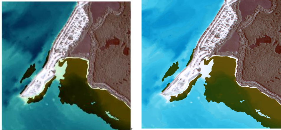
Figure 7. Synthetic images of the Sebastian Inlet area generated using the Monte Carlo model (left) and using the analytical model (right) using assigned bottom reflectance ( R_b ) data as SAV bottom reflectance (Bostater, 1992). Bathymetry data used was from SJRWMD. The depth in this area is between 0-5 meters. The water column is assumed to be pure water (no chemical constituents). The dark area near the shoreline is submerged aquatic vegetation (SAV). Images have been contrast stretched and do not include water waves influences. In general, the realism of the imagery begins to be seen when realistic bathymetry is used. Next, the realism is improved by the inclusion of realistic bottom reflectance of the known features or targets. For example below is shown the effects of simulating the geographical region indicated, but where a line target has been inserted as well as showing the influence of a realistic water wave surface.
