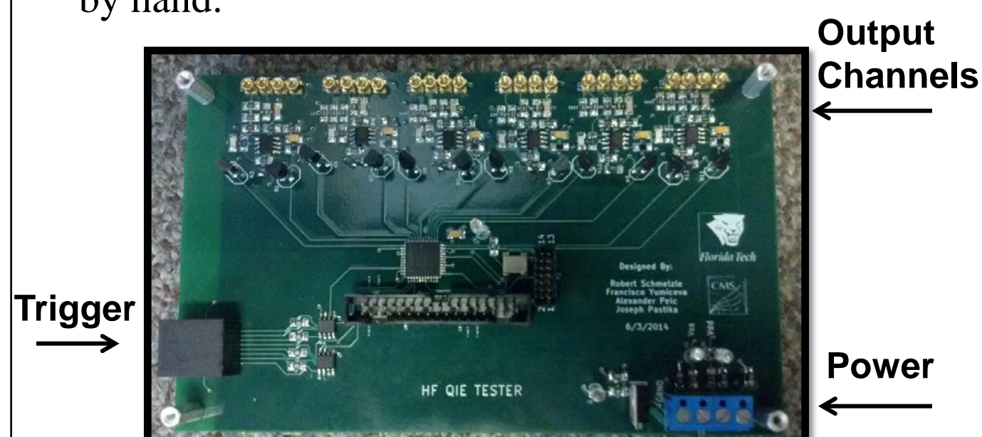
Figure 3: The Board – The completed board with six of the twelve sub circuits visible on the top.
