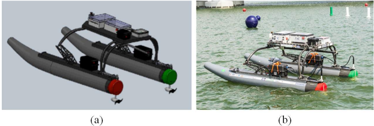
Figure 1 - The USV16 CAD model featuring the novel propulsion system (a). The USV16 in transit in Marina Bay, Singapore during the Maritime RobotX Competition
