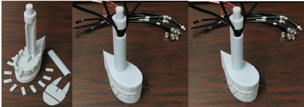
Figure 2: The modular design of robotic foil can incorporate up to twenty IPMC sensors and nine pressure sensors. Current work uses an array of eight IPMC sensors installed below an array of four pressure sensors. Wires are routed inside the body to maintain the streamlined foil shape of the prototype and limit un-modeled viscous effects [1].
