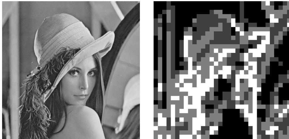
Figure 3. Left, original Lena 512×512 image. Right, classification map with 4 classes. Grey levels from dark to bright represent the “smooth area”, “mild change area”, “textures”, and “edges”, respectively.
