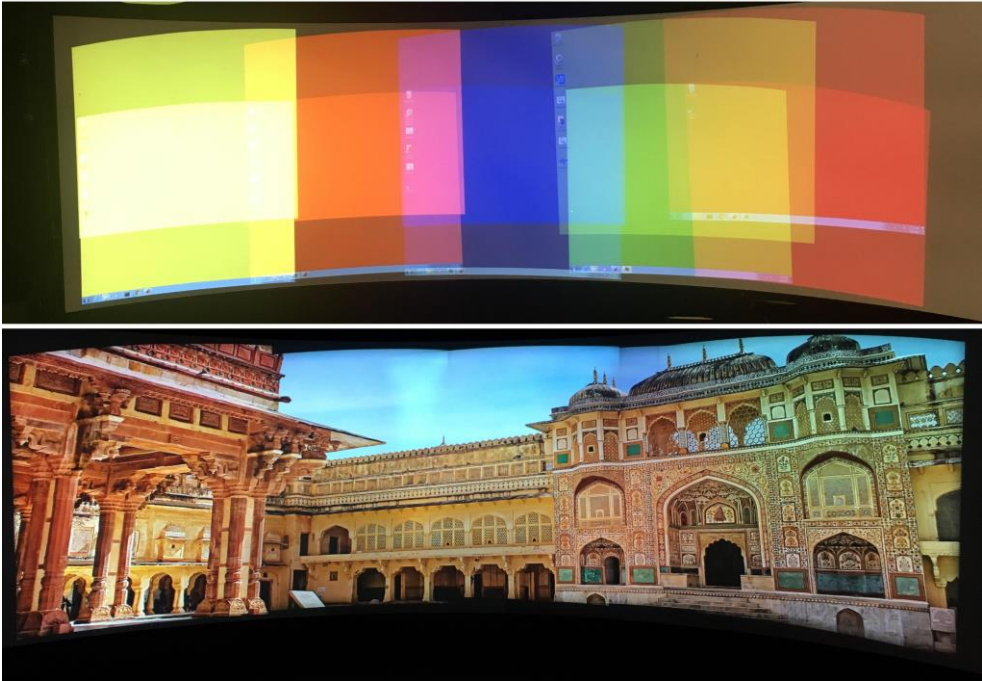
Figure 2 Our result of projecting on a half cylinder using 10 projectors and 4 cameras.
