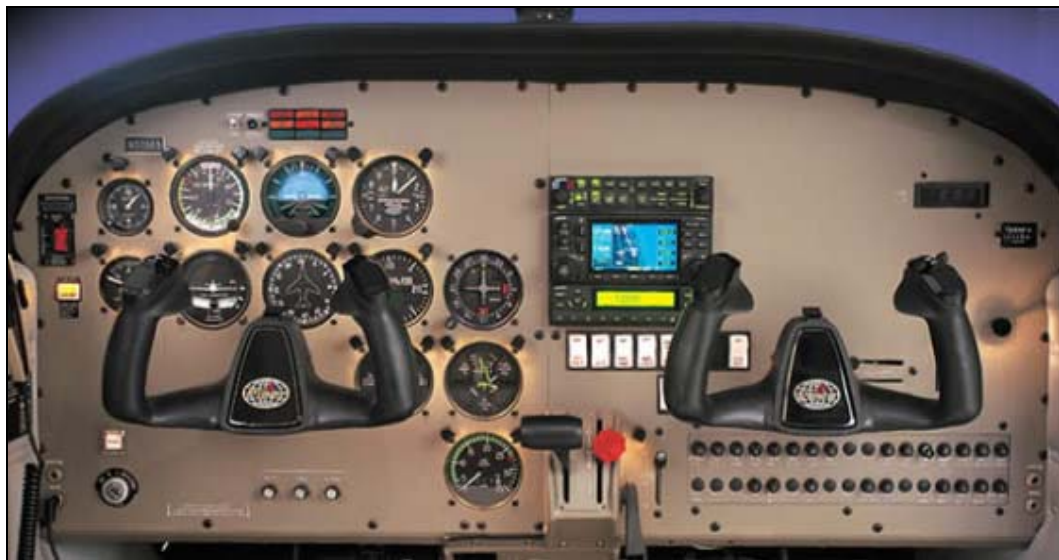
Figure 1. Conventional steam gauge cockpit
