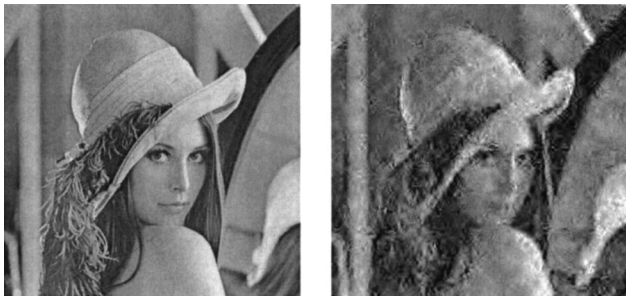
Fig. 6 Left, the “Lena” 512 image, and right, the reconstructed image based on original SPIHT when a single error occurs at the 10,000th bit. PSNR=22.22 dB.
