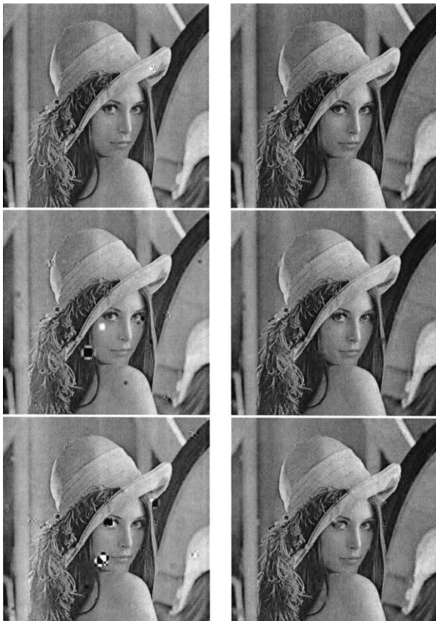
Fig. 7 Samples of reconstructed images over BSCs with BERs of 10^{-4} , 5 \times 10^{-4} , and 10^{-3} , respectively. The stop bit layer is 3. Left column shows images without error concealment and PSNRs of 33.92, 29.57, and 27.81 dB. Right column shows images with error concealment and PSNRs of 34.83, 32.69, and 31.37 dB.
