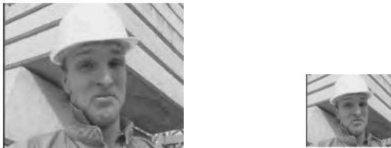
Figure 6: The right frame is decoded in 1/4 QCIF format from its corresponding frame in the left in QIF format.
