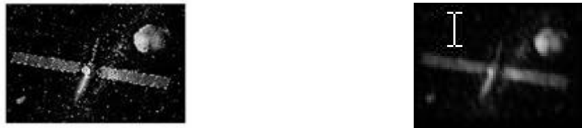
Figure 2: Left is the un-aberrated reference object brightness. Right is the aberrated image generated using the 4 th through 6 th Zernike polynomials all weighted by 2 radians.
