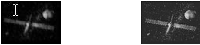
Figure 6: The left figure shows the aberrated image using the 4 th through 6 th Zernike polynomials. The right figure is the “corrected” figure using the phase diversity technique implemented with the CNN simulator.
