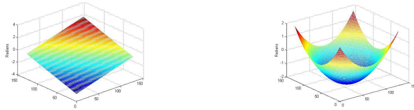
Figure 1: Zernike polynomial generated entrance pupil phases. The left figure shows the phase of an x -tilt and y -tilt with amplitude of 2 radians. The right figure shows the Zernike polynomial generated phase for the defocus term weighted with amplitude of 2 radians.
