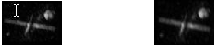
Figure 4: The figure on the left is the in-focus blurry image aberrated with Zernike coefficients 4 through 6. The right figure is the blurry image aberrated with Zernike coefficients 4 through 6 with an additional unit amplitude defocus term.
