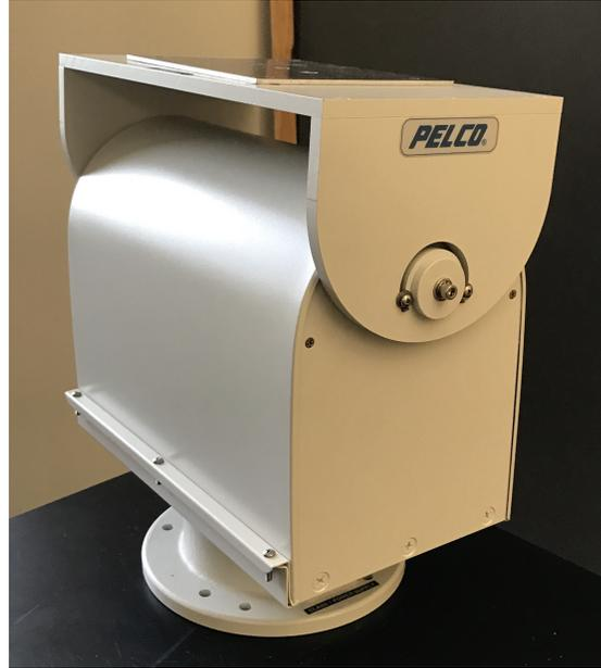
Figure 6.15: Heavy-duty Pelco motor for positioning the high-speed spectrograph.
