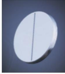
Figure 6.8: The optical slit used for the high-speed spectrograph.
