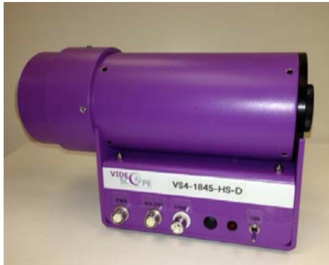
Figure 6.5: VideoScope VS4-1845-HS-D image intensifier.
