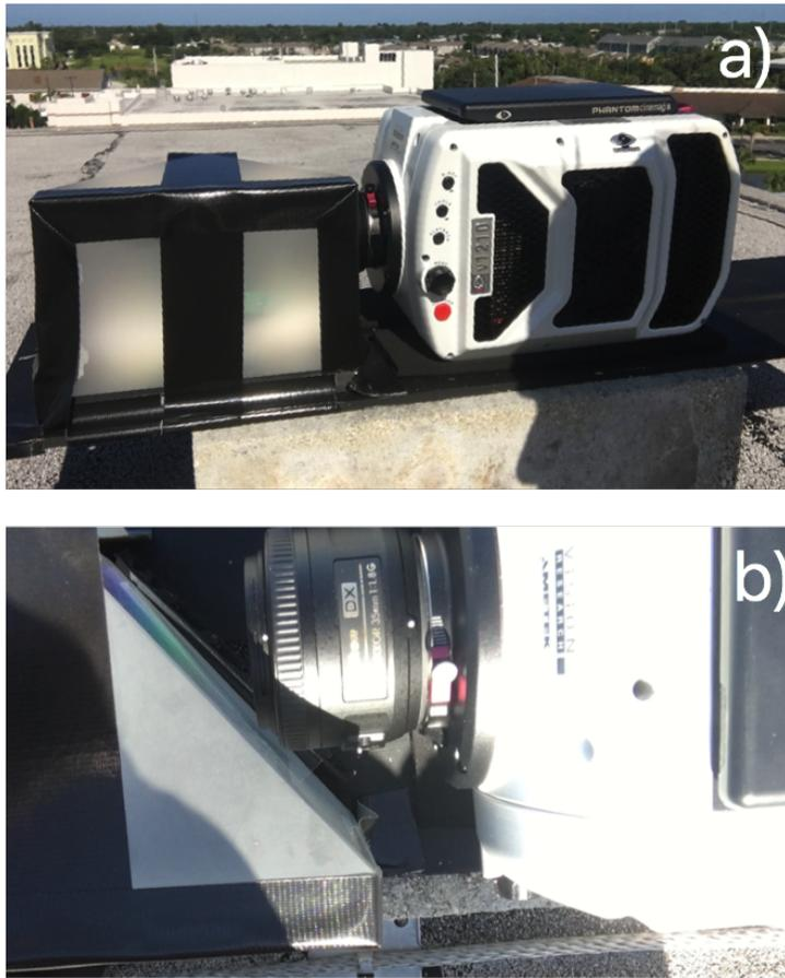
Figure 6.7: a) Side view of the high-speed camera and VPH grism mounted on the enclosure tray. b) Top view of the front lens of the high-speed camera and the VPH grism.
