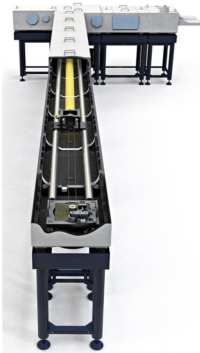
Figure 3.1: A Bruker IFS 125 HR. Projecting out of the page is the long ‘scan’ arm of the interferometer, on which a moving mirror is able to travel along the observed track. Perpendicular to the scan arm is a second arm that houses the infrared light source, the filled gas cell, and the detector. This image and more information about other Bruker instruments can be found on their main website: [www.Bruker.com](http://www.Bruker.com).
