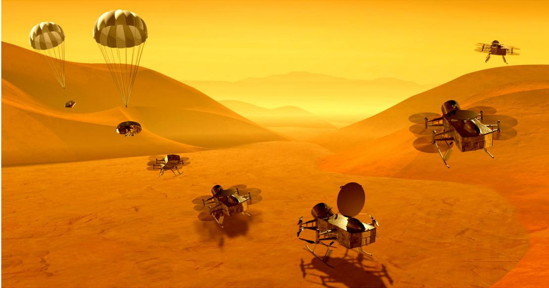
Figure 1.6: The Dragonfly rotorcraft, shown in stages, parachuting down through the Titan atmosphere before activating its propellers for a soft landing. Dragonfly will then fly to dozens of different nearby sites to study Titan’s surface and lower atmosphere.
