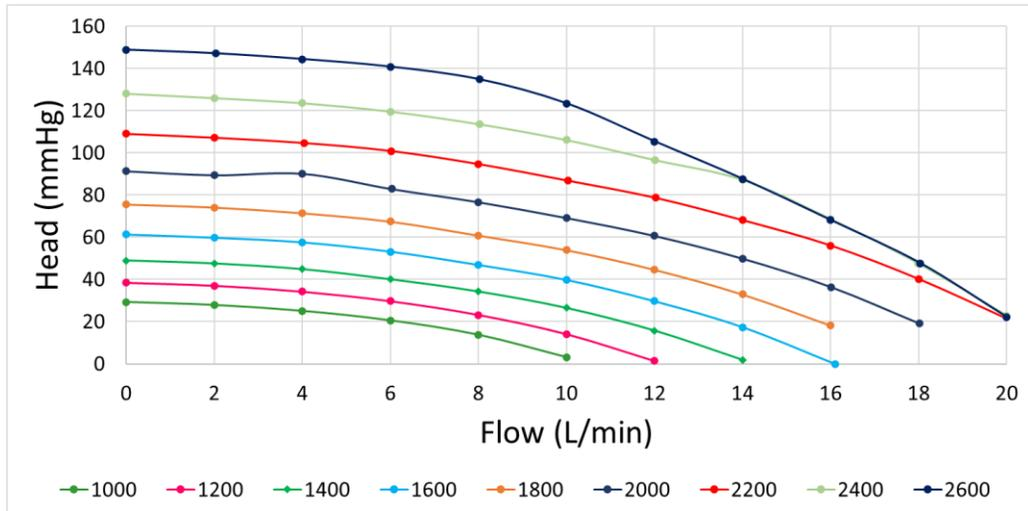
**Figure 42: The pressure flow curves for the EVAHEART 2 device**
