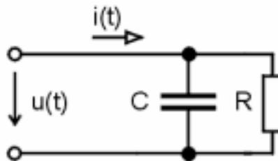
**Figure 8: Two-element Windkessel Model**<sup>51</sup>
