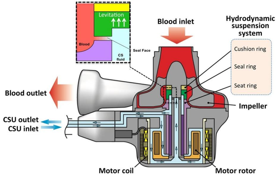
**Figure 6: The cross-sectional schematic view of the EVAHEART 2 hydraulically levitated impeller<sup>30</sup>**
