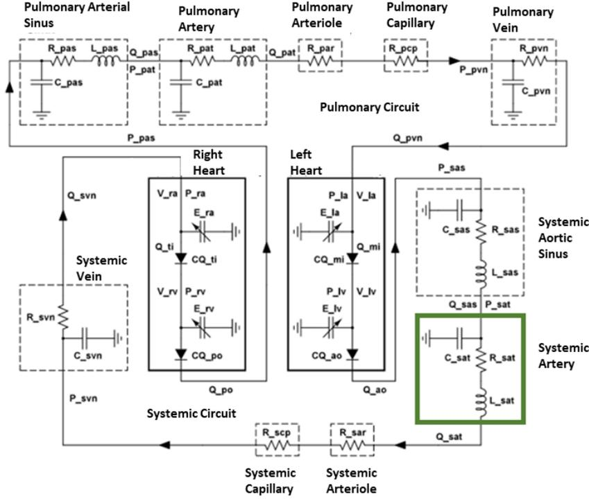
Figure 11: The lumped parameter model with its electrical components.<sup>52</sup>
