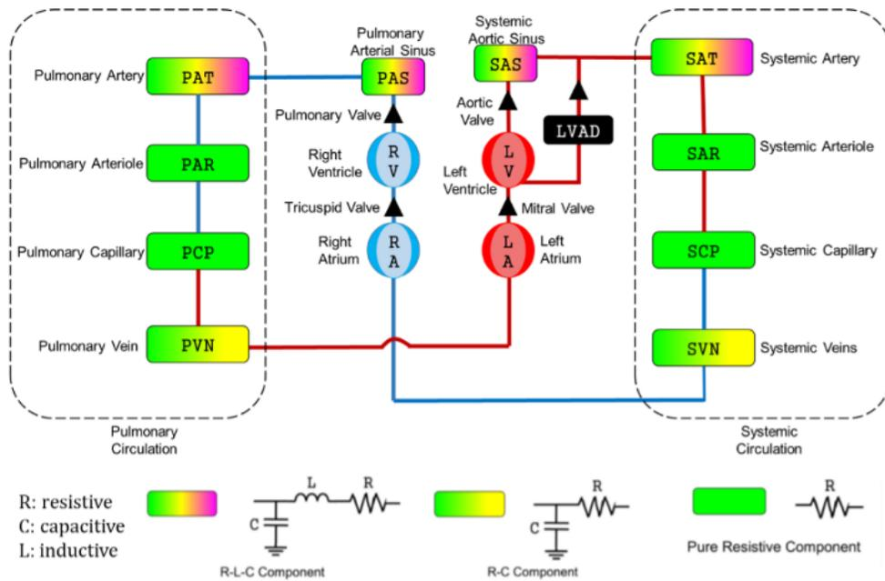
**Figure 17:** This figure shows the lumped parameter model in its entirety including the systemic and pulmonary circulations, LVAD support, as well as the pulmonary and systemic arterial/aortic sinuses, the four chambers of the heart, and the four valves.
