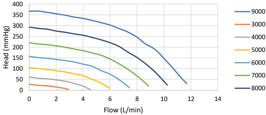
Figure 30: The pressure flow curves for the HM3. Speeds shown in the legend are in RPM
