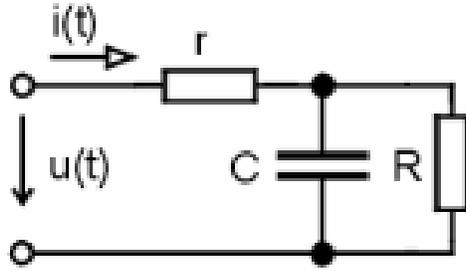
**Figure 9: Three-element Windkessel Model** <sup>51</sup>
