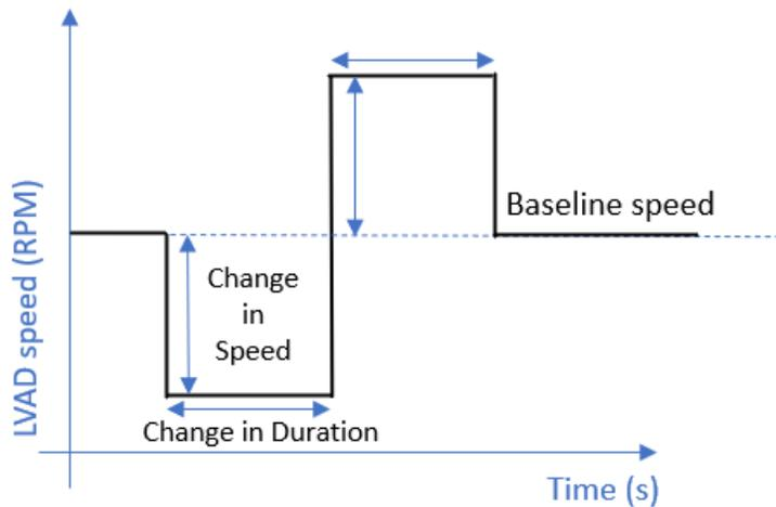
**Figure 38: The square wave speed modulation waveform**
