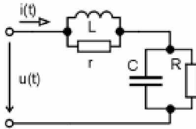
**Figure 10: Four-element Windkessel Model** <sup>51</sup>
