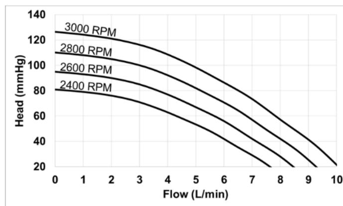
**Figure 22: Schematic of LVAD pressure-flow characteristics (Courtesy of Medtronic).**
