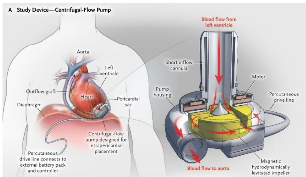
**Figure 3: The Heart Ware ventricular assist device system is shown**
