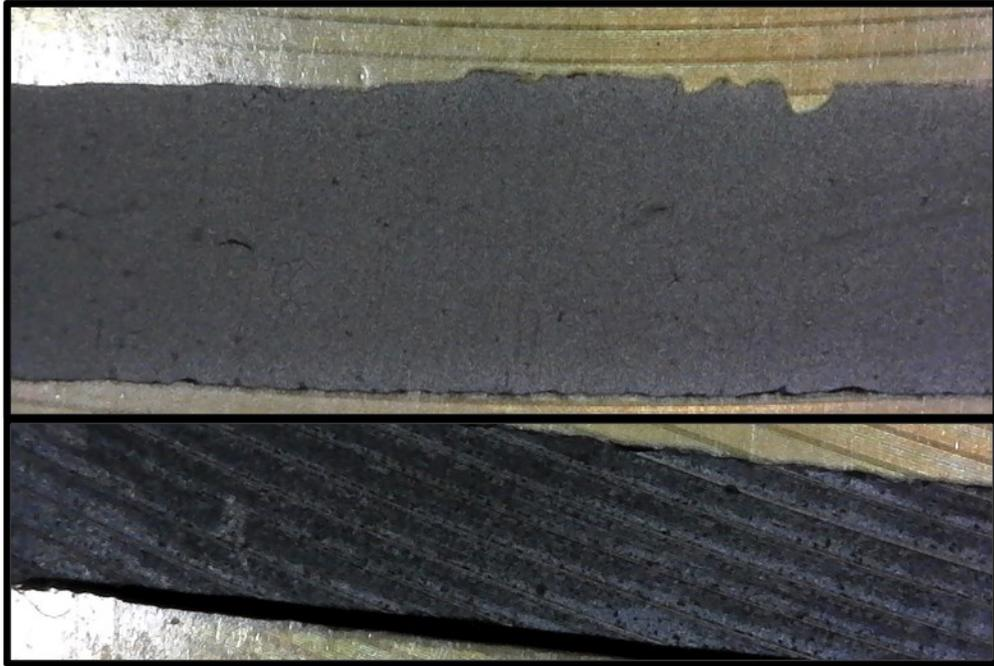
**Figure 9: Sample of the dried solution of Graphene oxide on the DVD disc (Top) and resulting laser scribed graphene (LSG) sample (Bottom)**
