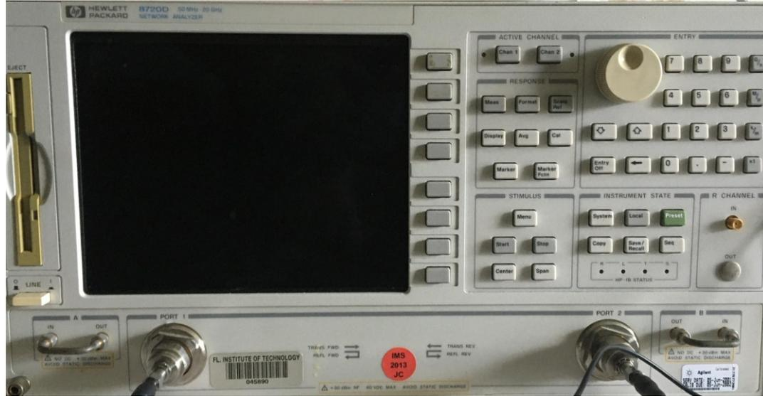
Figure 13: HP8720D Vector Network Analyzer
