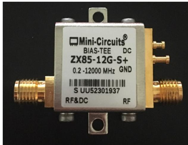
**Figure 12: Bias Tee used to input both RF signal and DC bias voltage as well as isolate DC bias voltage from the VNA**
