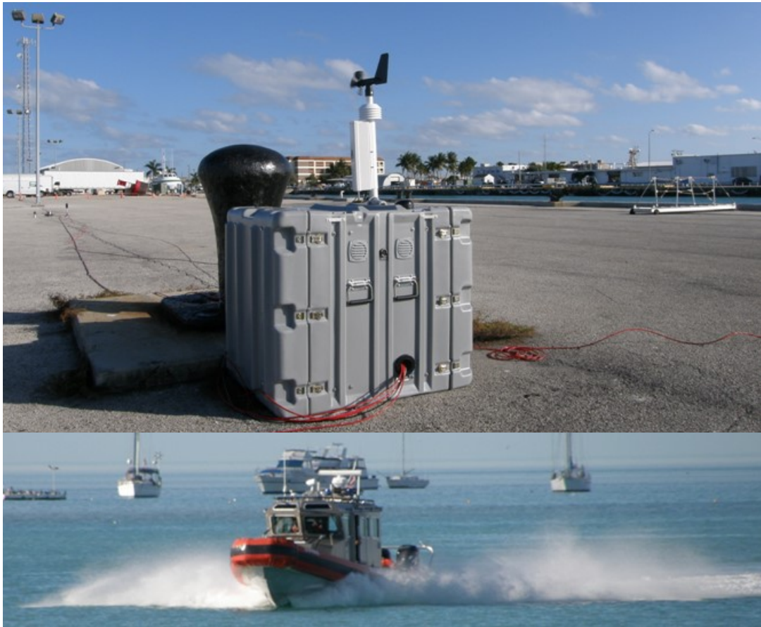
Figure 5-3 USCG Boat Experiment – Infrasound/Seismic Sensor Deployment (top) & Test Boat (Bottom) Used as Part of Field Experiment Conducted in Key West Fl. December, 2010 [Coots, et. al, 2016]
