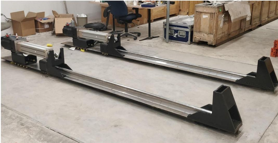
*Figure 25: Foundation with Linear Rails Mounted and Secured*
