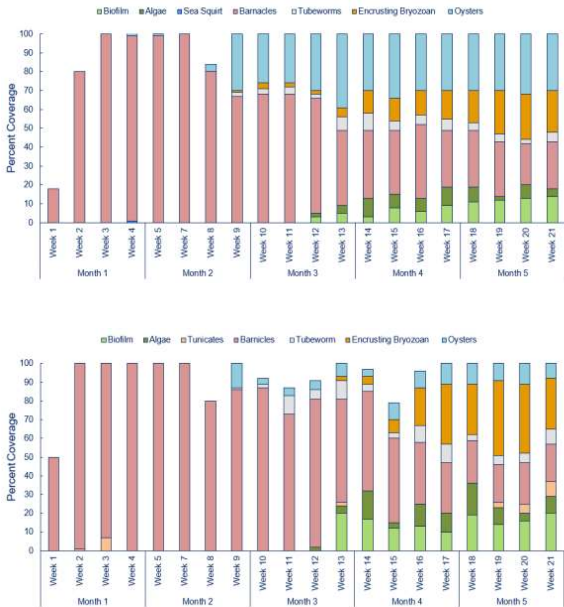
Figure 4.11. Percent cover of benthic organisms attached to steel mats (top) and plastic mats (bottom) at Melbourne Beach over a 21-week immersion period (Note: Week 6 assessment was not performed due to Hurricane Dorian).
