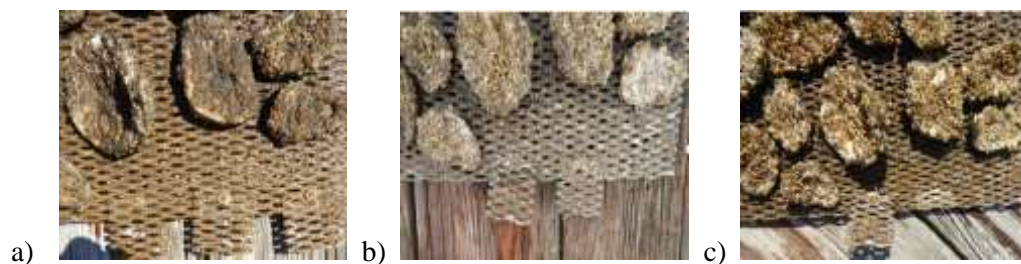
Figure 4.3. Examples of the sacrificial coupons after a) month one, b) month two, c) month three.
