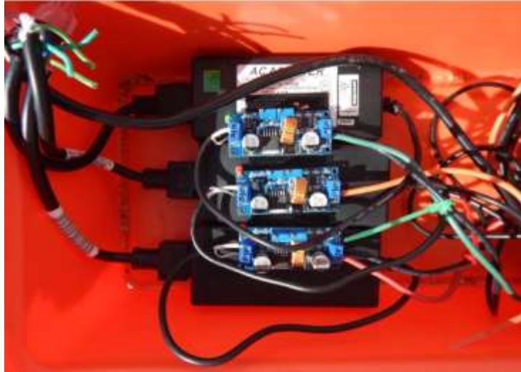
Figure 3.3. Power source setup for three different currents.
