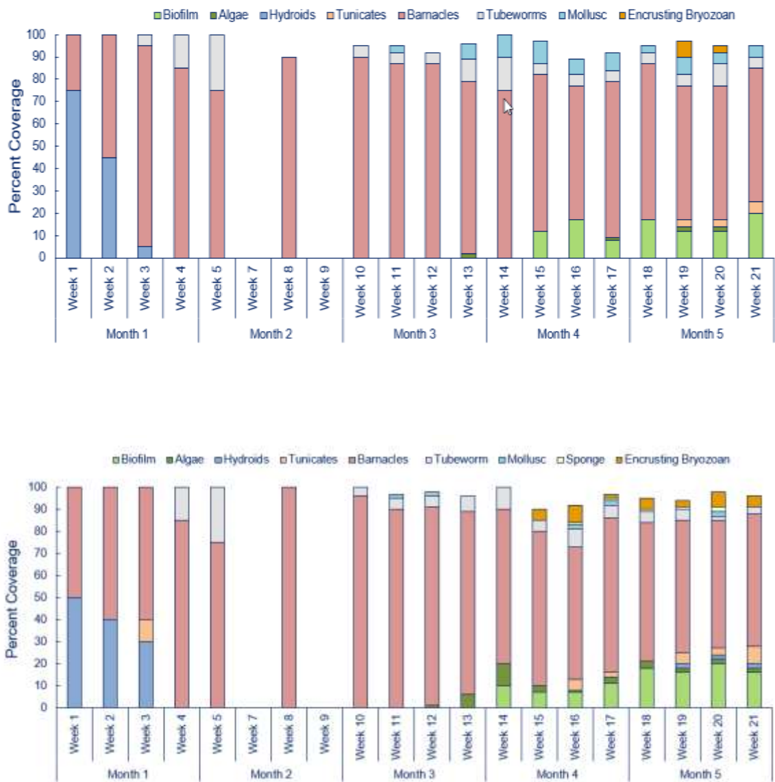
Figure 4.12. Percent cover of benthic organisms attached to steel mats (top) and plastic mats (bottom) at Grant over a 21-week immersion period (Note: Week 6 assessment was not performed due to Hurricane Dorian and Week 9 was not performed due to repairs).
