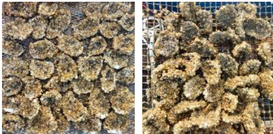
Figure C1. Oyster mats after month one immersion. Steel (left) and plastic (right) mats: a) Port Canaveral, b) Melbourne Beach, c) Grant.
