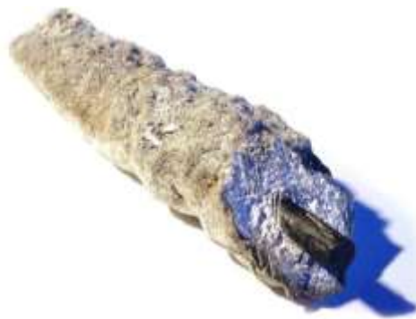
Figure 1.1. Biorock materials grown at Ihuru, North Male Atoll, Maldives. The steel is cathodically protected to prevent corrosion and allow for the buildup of mineral accretion (Goreau 2012).
