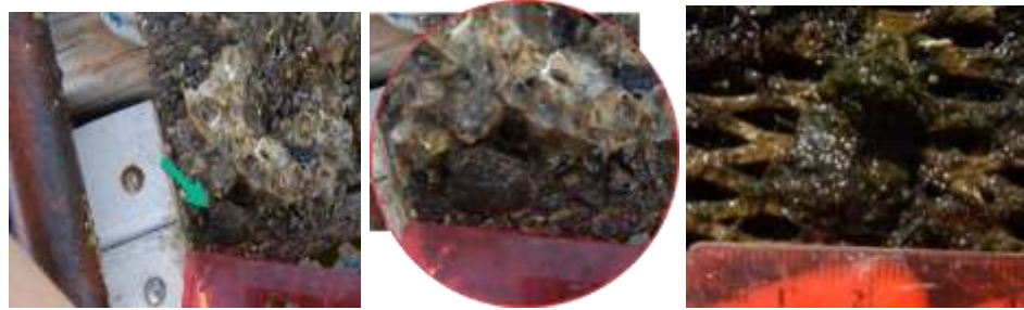
Figure 4.13. Photographs of oyster settlement directly on the steel mats: front of the mat (left), close -up (center) and back of the mat (right).
