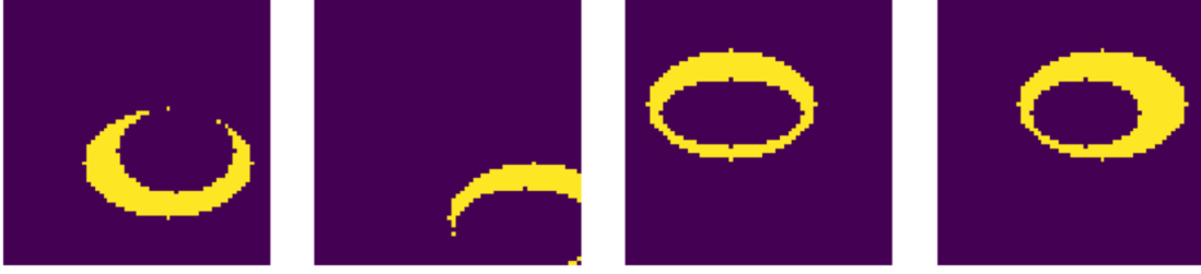
Figure 4.12: Annular elliptical rings. They are generated by two ellipse functions. The outer ellipse is fixed. By changing the center, the width and the height of the inner ellipse, we get different images to simulate hearts.
