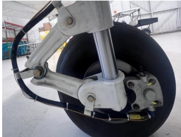
Figure 7 Backing plate and pressure plate thermocouple wires.
