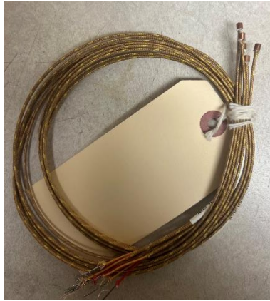
Figure 4 Shows K type thermocouple used to measure temperature of the back and pressure plate.
