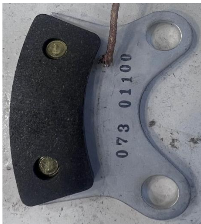
Figure 5 Pressure plate with thermocouple installed.
