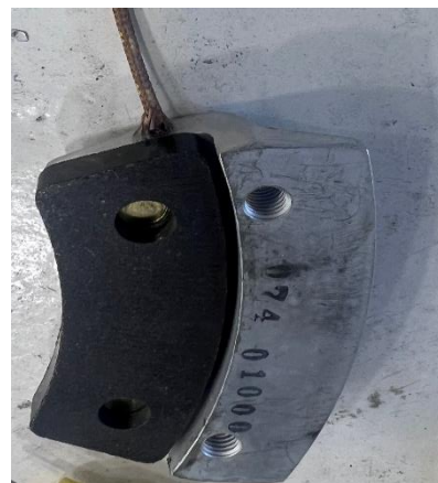
Figure 6 Backing plate with thermocouple installed.
