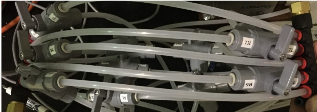
Figure 33 — Picture of port manifold system to direct static ports to differential pressure transducer
