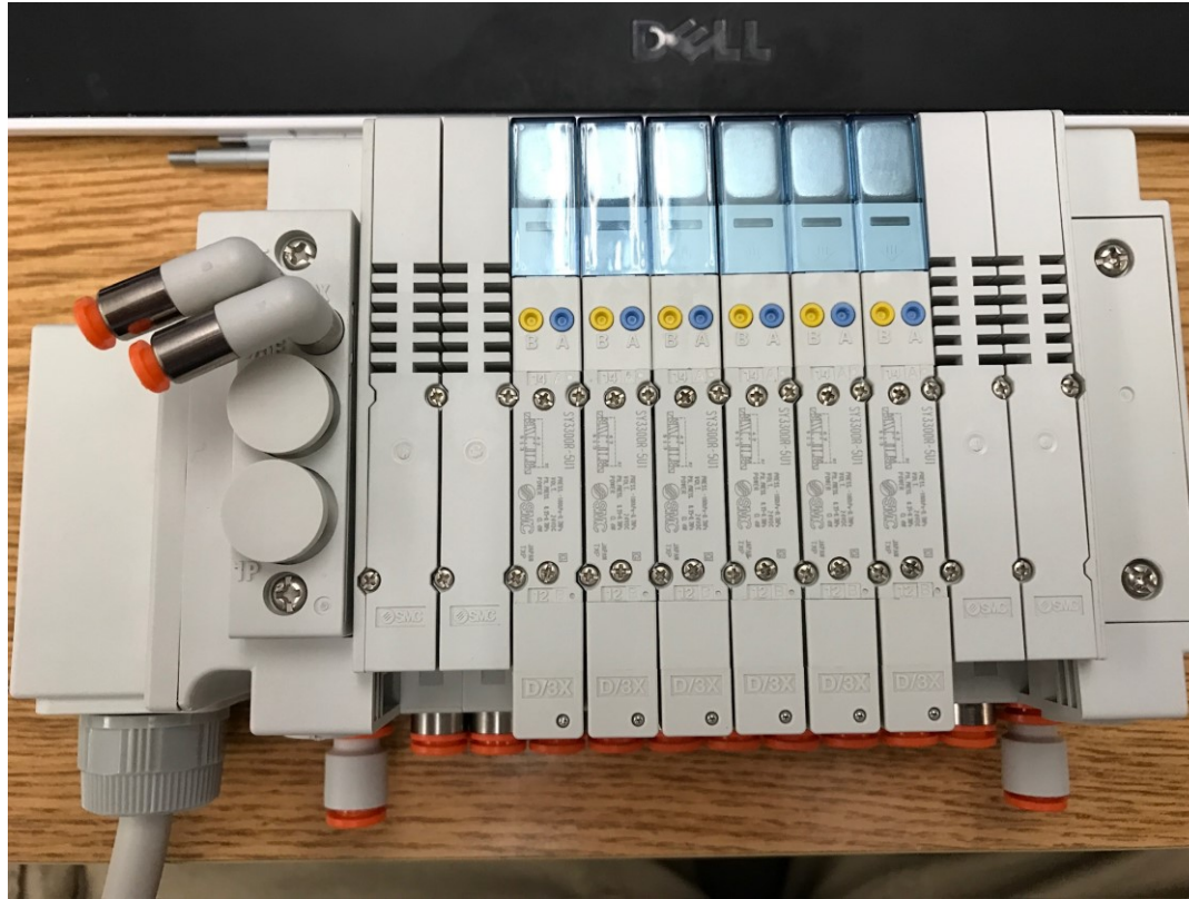
Figure 36 — Picture of automated valve switching system
