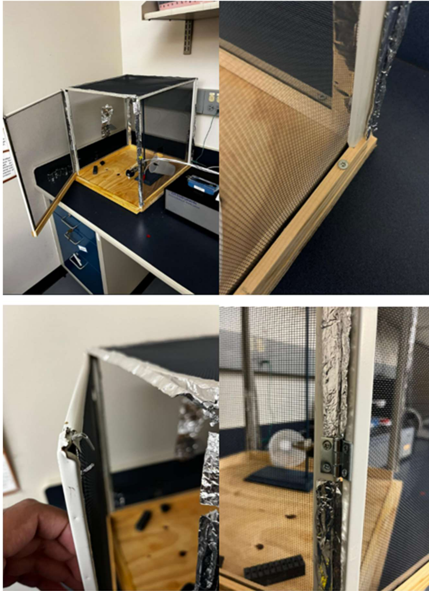
Figure 48 Images of the constructed Faraday cage.
